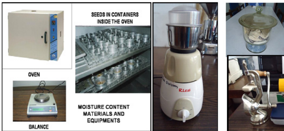
Figure : Accessories and equipment for seed moisture testing using oven method
