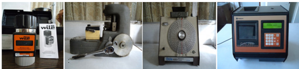
Figure : Different types of electronic moisture meters used in Seed Testing Laboratory
