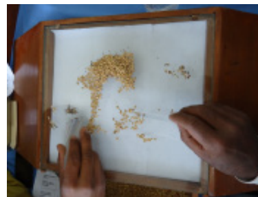
Figure: Purity testing of wheat on purity board
